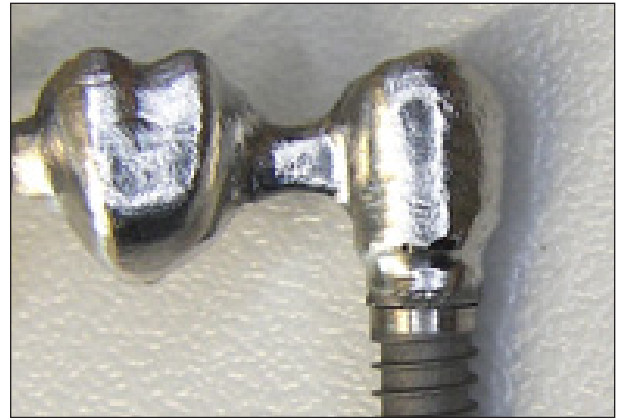
Fig 2 Casting imperfections have created a gap that is visible macroscopically (groups A and B).
